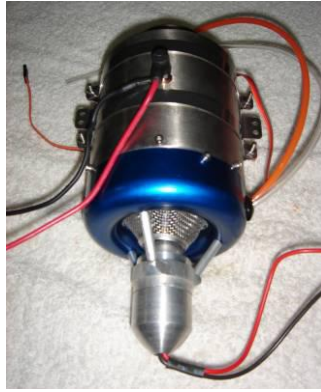
JJ 1400 in the Full-Auto configuration ready to go! (Temp probe not shown)
